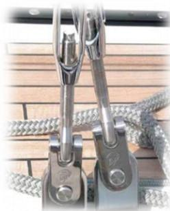
\*Use fresh water to rinse salt spray off accessible stainless steel rigging and lifelines after returning from sailing each time (just as you would your stanchions and pulpits)
