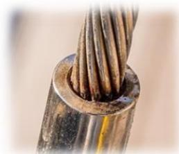
\*Look for spots with discoloration or rust as a crack in the stainless will generally promote rust. Any areas showing signs of rust should be thoroughly cleaned, polished and inspected to confirm there are no hairline cracks, or crystallization of the metal.
